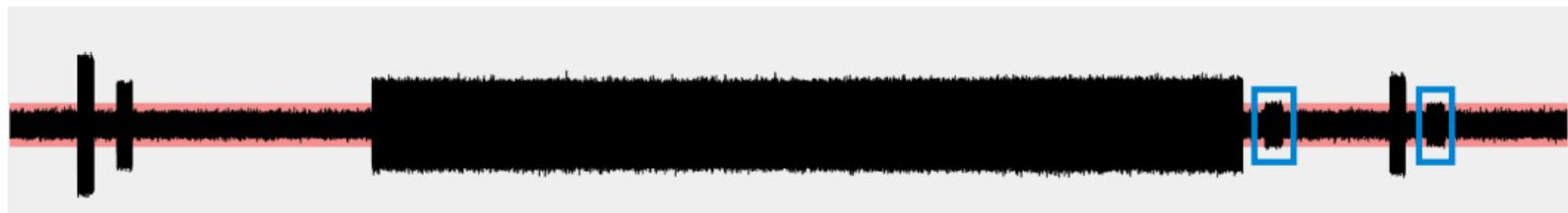
(b) Noise with 20% amplitude of mean signal power added
