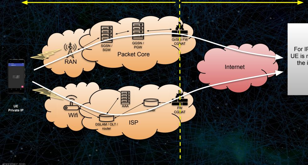
For IPv4 it is common that the UE is not directly reachable from the internet and it is located behind the NAT
