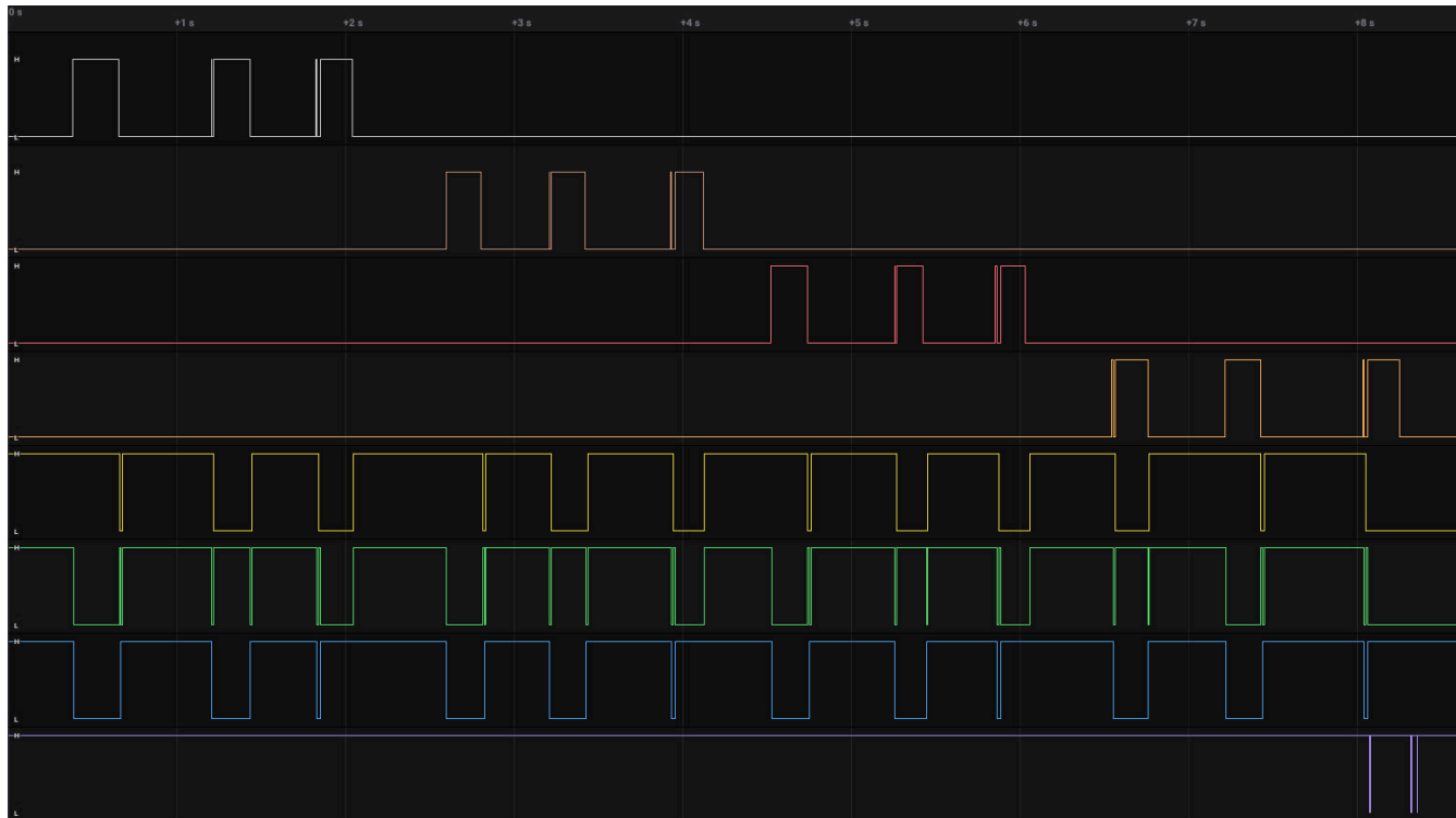
Encoding of all possible keys of the keypad
