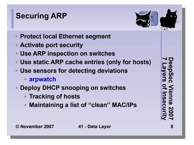
*Important note*: Some OS variants allow ARP packets to overwrite static ARP entries. Therefore static ARP entries should be taken with a grain of salt. Make sure your network code really does what you expect it to do.
