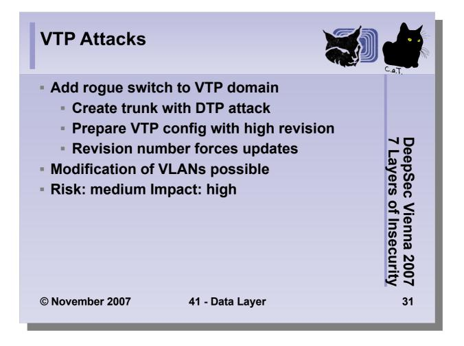
The mitigation of these attacks is the same as for DTP attacks. The guidelines apply to standard administration tasks as well. Be very careful when inserting new switches into your existing configuration.
