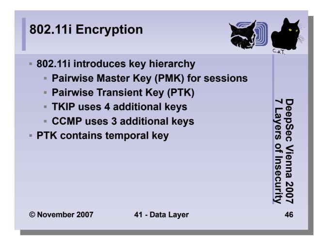
802.11i tries to minimally expose the PMK, because this key lasts for the whole session. The PTK is generated from PMK, AP nonce (ANonce), STA nonce (SNonce), AP MAC address and STA MAC address. All pieces are then processed by a cryptographic hash function. The generated PTK is then divided into 5 separate keys.
