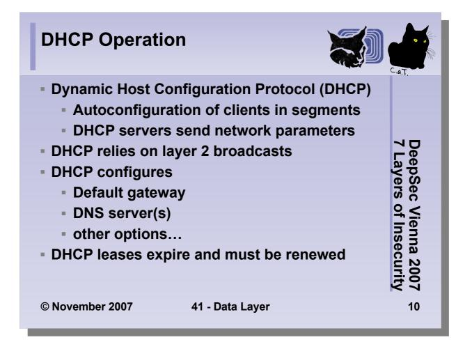
DHCP traffic can be transported between broadcast domains by use of DHCP Relay Agents on routers. These relay agents may increase the attack surface of DHCP servers assumed to be confined to Ethernet segments.
