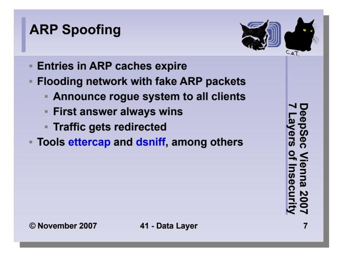
Ettercap allows for "port stealing" in a switched environment by using specially crafted ARP packets. The authors of the software describe the techniques in their presentation slides (showed at Black Hat 2003).
