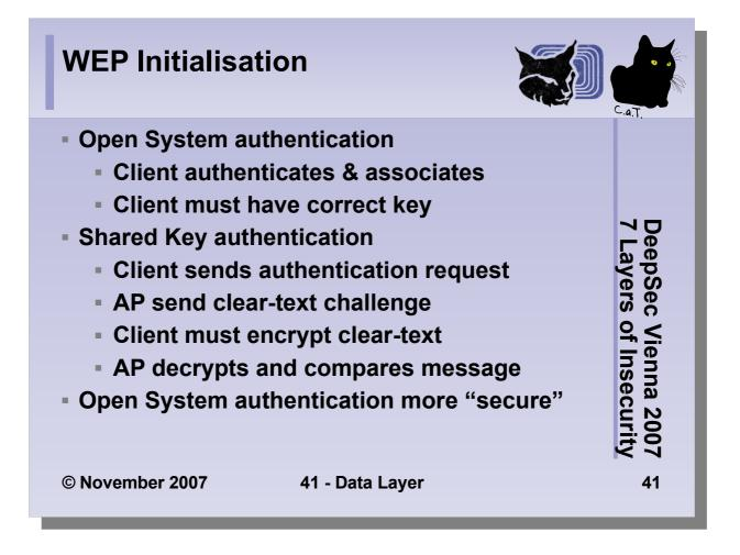
The shared key authentication has a major drawback. Provided an attacker can capture the packet exchange used for authentication, then two out of three pieces of information of the whole WEP security is known. The packets contain the clear text challenge string and what the challenge string looks like after it has been encrypted. Together with the RC4 encryption algorithm the attacker can deduce the shared authentication key which in turn is used for WEP itself.
