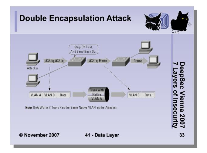
The graphics shows the double encapsulation attack. The attacker creates Ethernet frames with two VLAN tags and sends them to a switch. The switch strips the first tag and forwards the frame to the VLAN indicated by the second tag. The attack only works if the trunk has the same VLAN ID as the attacker.
