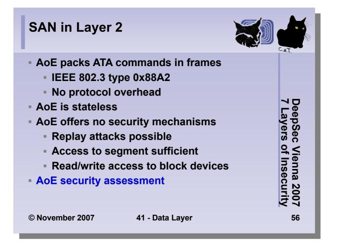
AoE is a typical internal protocol and is part of the infrastructure. It is not designed to provide strong protection. This is true for other protocols used for providing direct access to resources with low overhead (i.e. no protection).
