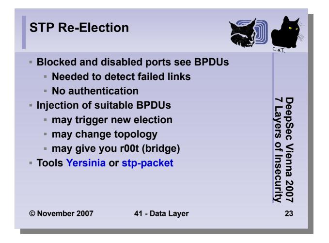
The tools Yersinia and stp-packet give you the possibility to inject crafted BPDUs. The packets must be created manually and must fit into the existing topology in terms of bridge IDs.
