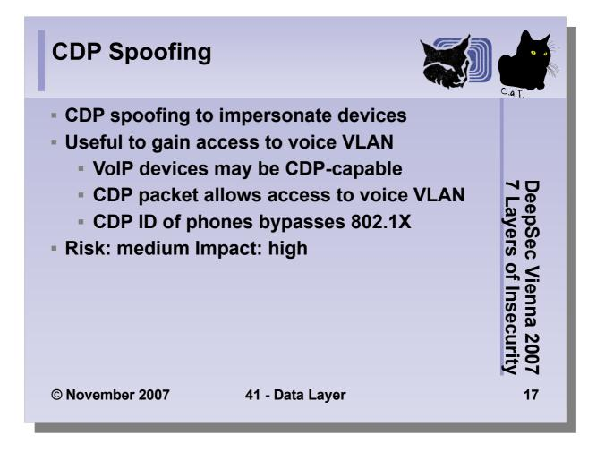
The CDP spoofing vulnerability was published by FishNet Security in 2005. They tested Cisco IOS and CatOS versions in combination with a VoIP setup consisting of CDP-capable IP telephones.
